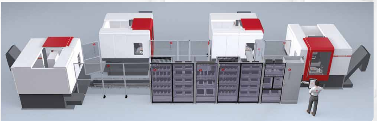
Numerous automation systems can be connected to the HEDELIUS ACURA range, such as multi-pallet storage systems in the Indumatik Light or Erowa Leonardo models, all the way through to linear systems for the chain-linking of several machines.
